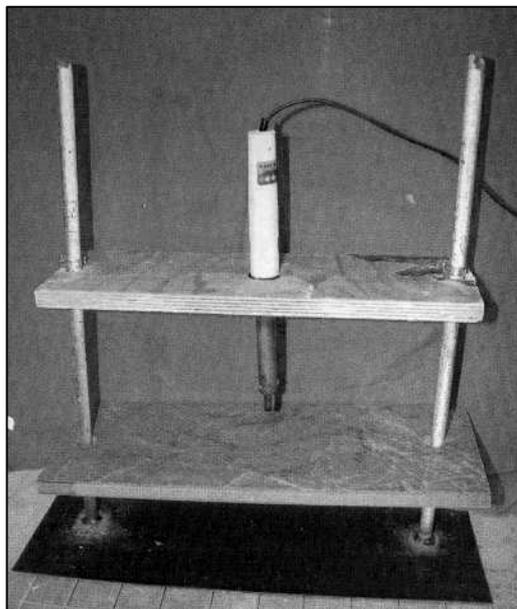
**Figure 1.** Customized frame to make a constant pressure of soldering iron. The rabbits were put on the lower plate. The upper plate was movable and adjusted so as the tip of iron just touched the skin.
