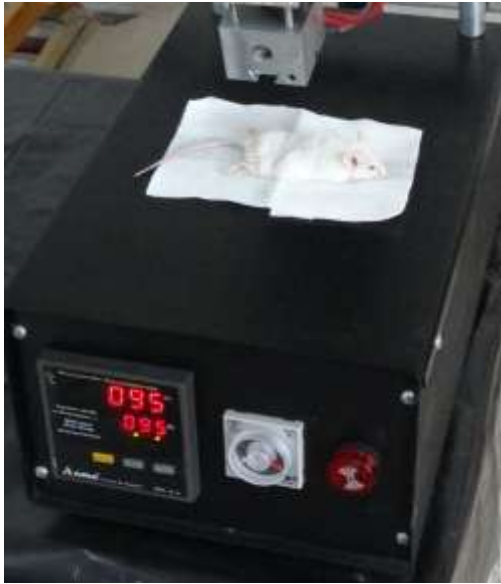
Figure 1: The device for skin burn induction is setup for 95° C and 10 seconds and the heated exchangeable iron plate is applying over mouse skin.
